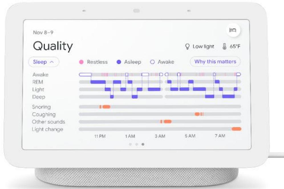
Google launched sleep sensing through the Nest Hub, its smart home controller, in 2021. Low-energy radar detects granular motion, while microphones and other sensors detect snoring, coughing, ambient light, and other factors.
